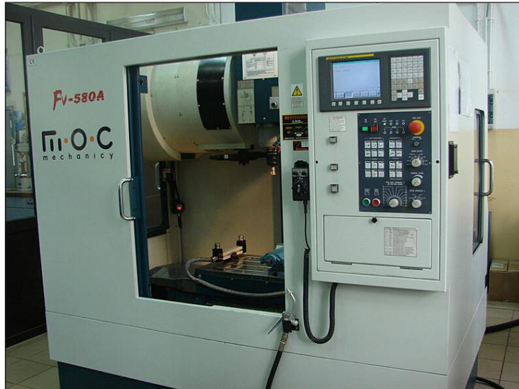
Fig. 2. MOC Mechanics FV580A machining centre
